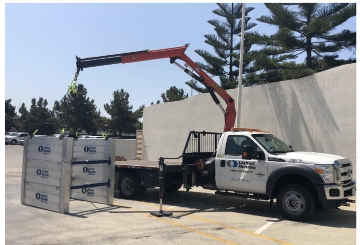
**Spreader bars should be used only to hold the box walls in place, not for pulling the box up or relocating it in any way.**
