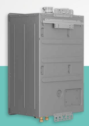
Rheem<sup>®</sup> IKONIC<sup>®</sup> can be installed either with direct vent (outside air) or non-direct vent (room air) intake. Room air intake allows maximum installation flexibility in an open area like a basement or garage, as well as in smaller spaces like a closet with full louvered door.
